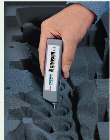
Battery-operated measuring instrument with digital readout for the determination mould strength of test specimens sand moulds.
