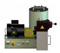
This mixer is designed to mix liquid binders with sand that is common to all chemically bonded sand mixtures. The mixer features an "S" shaped mixing blade with a vertical shaft that completely mixes the sand mass.
