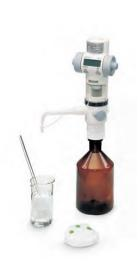
The Methylene Blue Clay Tester is used to determine the amount of live bentonite clay present in a sand sample. This instrument utilizes a magnetic stirrer for removal of the clay coating from the surface of the sand grains.
