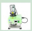
The Rapid Sand Washer is used to ensure correct and repeatable test results when preparing sand samples for the AFS Clay Tester (Model 42131). This sand washer uses highspeed agitation to remove all clay from the sand grains within the molding sand sample.
