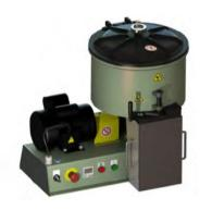
The Simpson Laboratory Muller is used to prepare mixtures of clay bonded foundry sands. The mulling conditions found in industrial mullers can be emulated on a smaller scale using this laboratory muller.
