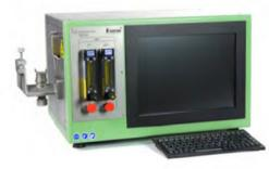
This tester measures the temperature at which shell resin coated sands melt and adhere to a heated bar. The melting temperature of the sand is considered the melt point or stick point.
