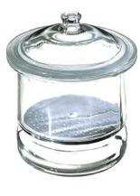
The desiccator is used to protect sand specimens from water vapor in the air during the cooling of samples after those samples have been heated in the Muffle Furnace (Model 42127).
