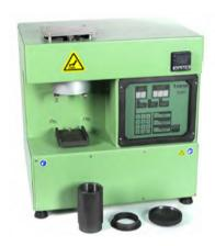
The tensile strength of the condensation zone in a clay bonded molding sand can be accurately measured using this technology. The automated instrument simplifies the testing process and displays the wet tensile results in an easy-to-read digital display.
