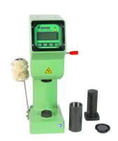
This sand squeezer is used to prepare standard AFS 2" x 2" (50mm x 50mm) sand specimens and to determine the compactability of prepared clay bonded molding sand. The instrument can be a replacement for the standard 3-ram method of making sand specimens using a traditional sand rammer.
