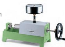
This hand-driven strength machine is used to determine the strength properties of clay and/or chemically bonded foundry sand specimens. The device has the capability to run five different sand strength tests with additional fixtures and accessories that are easy to connect to the instrument.
