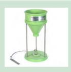
This accessory assists in filling the specimen tube for compactability tests. It assures that properly riddled sand fills the specimen tube from a standard and fixed distance. Both the Digital Pneumatic Sand Squeezer (Model 42160) and the Sand Rammer (Model 42100) use this accessory.
