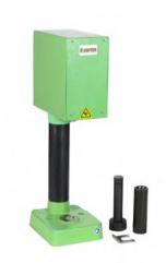
This instrument is used to prepare AFS standard sand specimens of clay bonded molding sand used for high temperature compression testing in the High Temperature Compression Tester (Model 42115).
