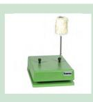
To ensure consistent and accurate readings, the Sand Rammer (Model 42100) needs to be isolated from vibration variations. This base is mounted to the rammer to achieve uniform ramming energy.
