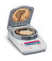
To determine the moisture content of green sand and other raw materials used within the foundry, this analyzer can be used.
