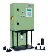
This multi-purpose instrument is used to determine strength properties of clay and/or chemically bonded sand specimens. The Minilab may be used to create a 50mm x 50mm cylindrical test specimen and can run many different sand strength tests using additional accessories. These tests include: compactability, compression strength, splitting strength, twin-transverse shear strength, core transverse (bending) strength and core tensile strength.
