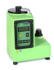
The Digital Absolute Permmeter measures the permeability of standard AFS 2" x 2" (50mm x 50mm) sand specimens. With the addition of optional accessories, this instrument can measure the permeability of unbonded sand, coatings, cores and molds.
