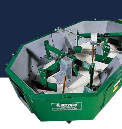
Based on sensors monitoring motor load, the control system adjusts the discharge door opening to maintain a constant volume of sand in the cooler at all times.
