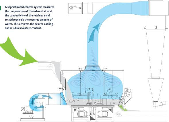
2 Counter-rotating mixing tool sets mechanically fluidize the retained sand so that cooling air, provided by the inlet blower, and water can be in intimate contact with the sand; thus providing for efficient and effective cooling.
