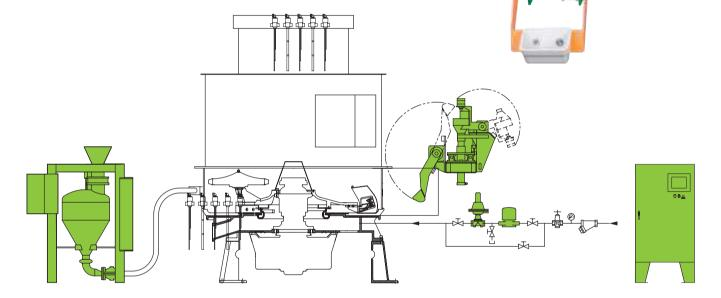
The data from each test (available for display or can be exported to a data system) on all model testers includes: time of day, test number, return sand temperature, return sand conductivity, target compactability, actual compactability, target water addition, actual water addition, maximum muller drive motor amperage, target bond weight, actual bond weight and compactability deviation. The model 2552 additionally provides green compression strength, available bond
