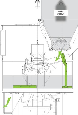
2 Interchangeable, modular plows armored with tungsten carbide provide intensive blending and minimize maintenance costs.
