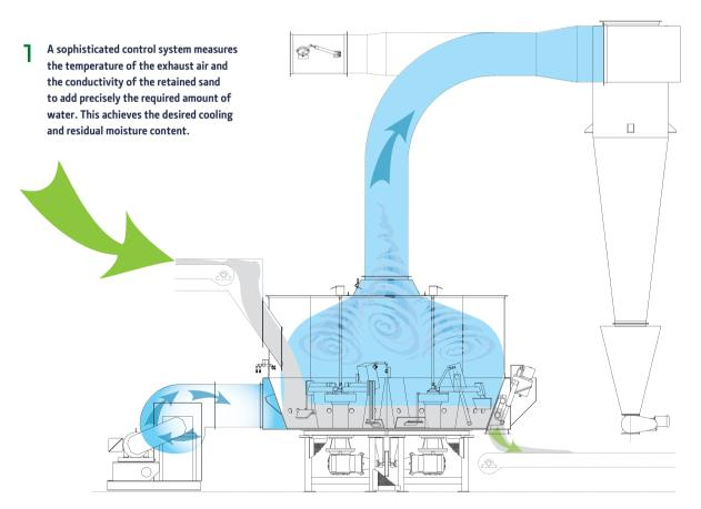
Counter-rotating mixing tool sets mechanically fluidize the retained sand so that cooling air, provided by the inlet blower, and water can be in intimate contact with the sand; thus providing for efficient and effective cooling. Based on sensors monitoring motor load, the control system adjusts the discharge door opening to maintain a constant volume of sand in the cooler at all times.
