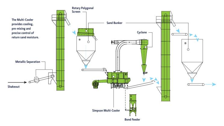
Simpson Multi-Cooler, in seven models, provides pre-mixing, cooling and moisture optimization before final mixing.
