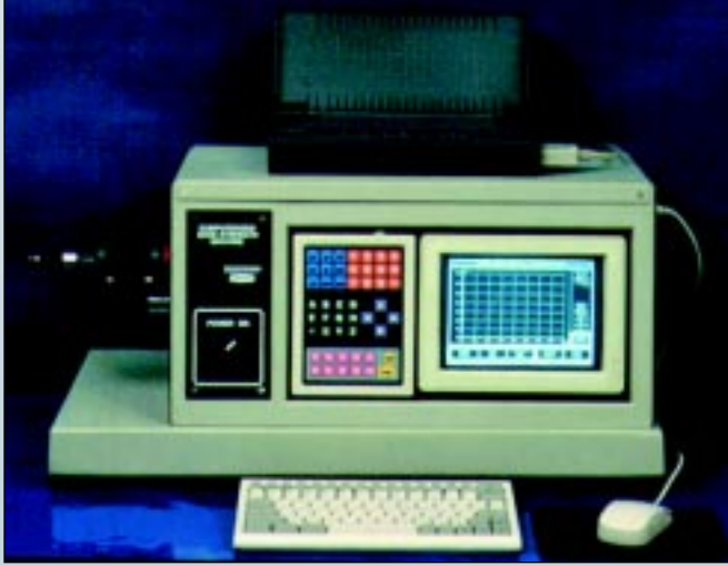
Fig. 3. This instrument, comprised of a hydropneumatic press, microprocessor, keyboard, monitor, displacement transducer and electronic load cell, provides the first accurate way to quantify a sand's flowability.
