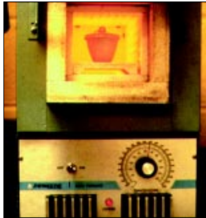
A volatiles test is conducted to determine the amount of live carbons in a sand system.
